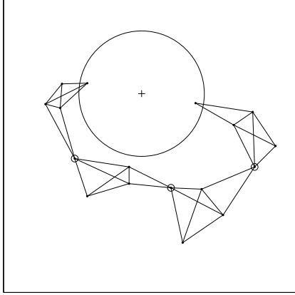
Fig. 5. An example of a connected network that can be made biconnected by adding a single relay node, e.g. at the point marked with the '+'-sign. The articulation points are circled.
