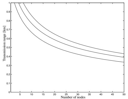
Fig. 1. The transmission range predicted to ensure  $k$ -connectivity with 99% confidence for randomly placed nodes in a  $1 \text{ km} \times 1 \text{ km}$  area. 3-, 2-, and 1-connectivity, from top to bottom.
