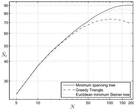
Fig. 7. Average number of relay nodes needed to connect the network, taken over 1000 random realizations and plotted on log-log -scale. The transmission range is 5% of the side of the domain. The Greedy Tessellation algorithm has been omitted for clarity.
