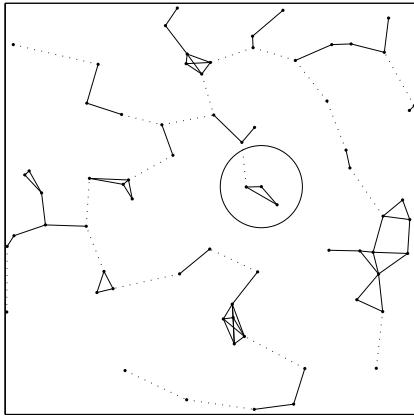
Fig. 2. Minimum Spanning Tree algorithm. The initial clusters in this example realization of 70 terminal nodes are connected with solid edges, and the edges to place relay nodes are dotted. The transmission range is 10% of the side of the domain, as illustrated by the circle.
