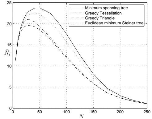
Fig. 6. Average number of relay nodes needed to connect the network, as a function of the number of terminal nodes initially in the network, taken over 1000 random realizations. The transmission range is 10% of the side of the square-shaped domain.
