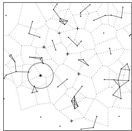
Fig. 3. An example of the Greedy Tessellation algorithm, when applied to the same realization as in Figure 2. The edges of the Voronoi tessellation are shown with dotted lines, the candidate points for relay node insertion with '+'-signs. The first location to add a relay node is marked with an asterisk.
